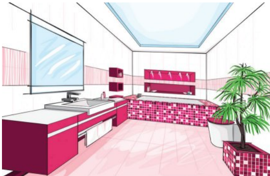
Figure 5.41 One-point perspective drawing of room interior
