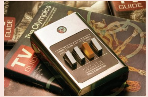
Figure 2.37 Zenith electronics corporation developed the world's first cordless television remote control in the 1960s
