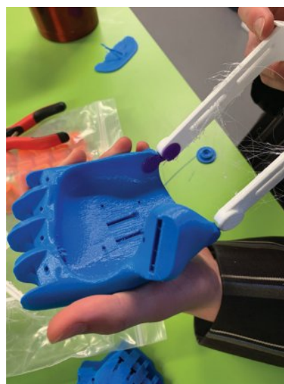
Figure 4.14 Tom Polizzi designed a prosthetic hand that was to be both affordable and more durable than the average prosthetic, to alleviate financial stress and provide long-term assistance to victims. The design also needed to be 3D printed, be able to be repaired and parts re-printed to prolong its use.
