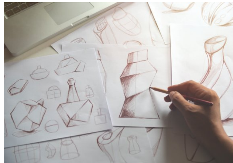
Figure 4.16 Freehand development drawings used during ideation. Initial industrial design drawings may be quickly generated with pencil or fine liner to allow continuous thought processes.
