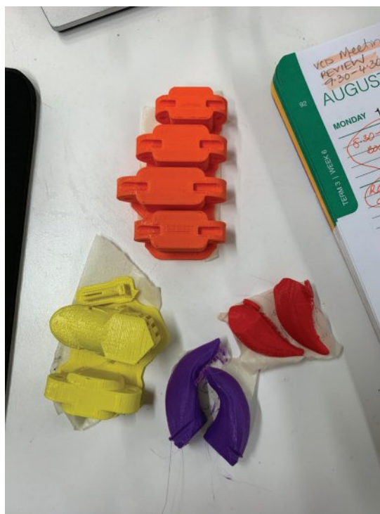
Figure 4.70 Manual low-fidelity prototyping; at this stage the colour and quality of 3D printing was not the primary focus. By Tom Polizzi
