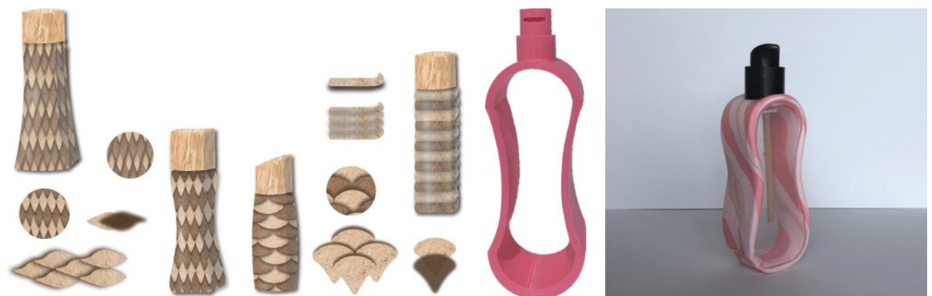
Figure 11.22 Alessia Wynne used both manual and digital model making to explore potential concepts. Left to right: digital models, 3D printed prototype and polyoma clay model
