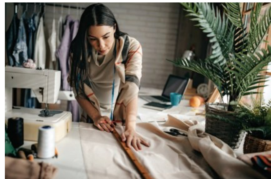
Figure 4.1 Zero waste sewing often uses written instructions rather than paper patterns and aims to create little or zero waste in the cutting of fabric. The process requires the user to follow instructions to draw the pattern pieces directly onto the fabric or paper if they want to create a paper pattern.
