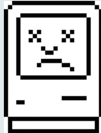
Figure 6.20 Susan Kare designed the 'sad Mac' icon, which appeared if a hardware or software problem was preventing computer startup.
