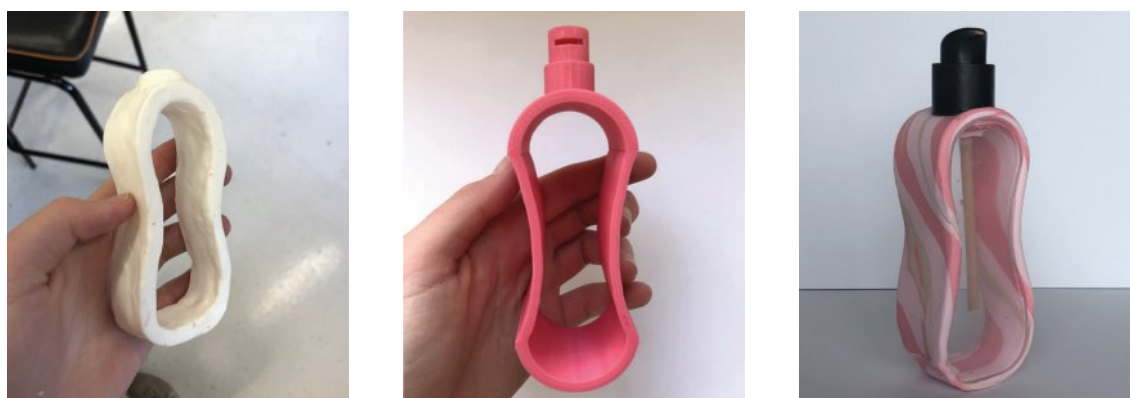
Figure 4.69 3D prototypes using different methods, media and materials. Left to right: resin, plasticine, and 3D printing. Prototyping was undertaken to resolve methods and materials for final presentations. By Alessia Wynne
